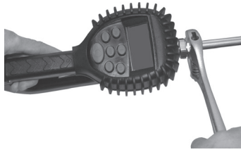
Figure 6: Tighten nozzle with wrench
