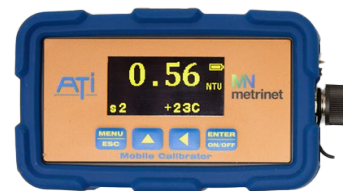
Figure 3: Q51 Calibrator for sensor
