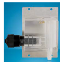
Figure 2: Constant head flow cell
