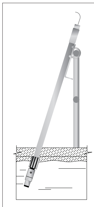
Figure 4: Sensor handrail mounting
