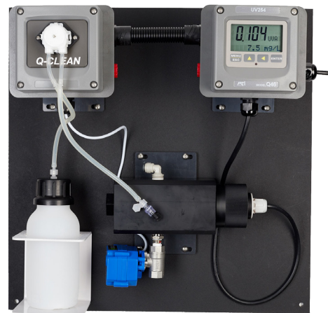
Figure 2: Automatic sensor cleaning
